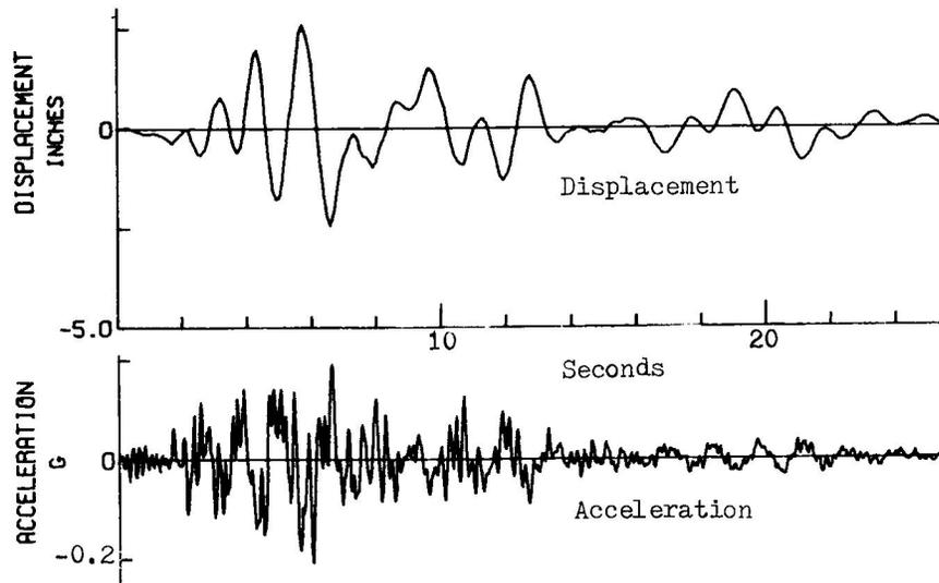
Figure 7b. Motion recorded on the roof of the 9-story steel-frame Jet Propulsion Laboratory Building during the San Fernando earthquake. This motion produced maximum stresses in the frame that almost reached yield point. The building suffered only minor damage, such as cracking of plaster partitions, cracking of concrete fireproofing, etc.
