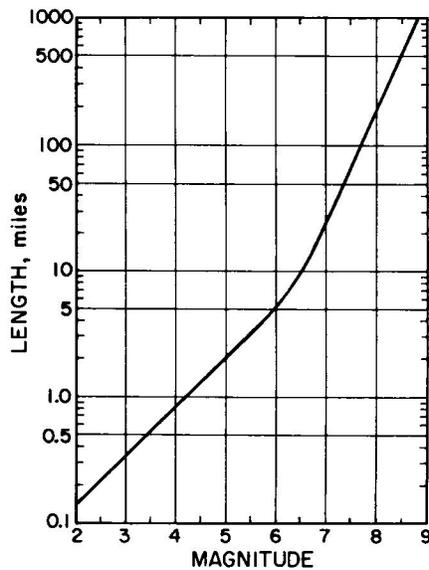
Figure 3. Diagram relating the magnitude of an earthquake with the horizontal dimension of the slipped fault area. This idealized diagram represents an average relation but is useful in estimating the surface area affected by earthquakes of different magnitudes.
