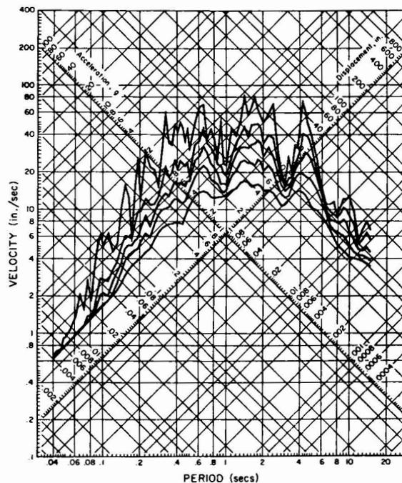
Figure 11. Response spectrum plotted on three-way log paper for the ground acceleration recorded at the Holiday Inn during the San Fernando earthquake, approximately 5 miles from the causative fault. For periods approaching zero, the spectrum curves approach the peak ground acceleration; and for very long periods the spectrum curves approach the peak ground displacement. (The spectrum curves are for 0, .02, .05, 0.1, 0.2 of critical damping.)
