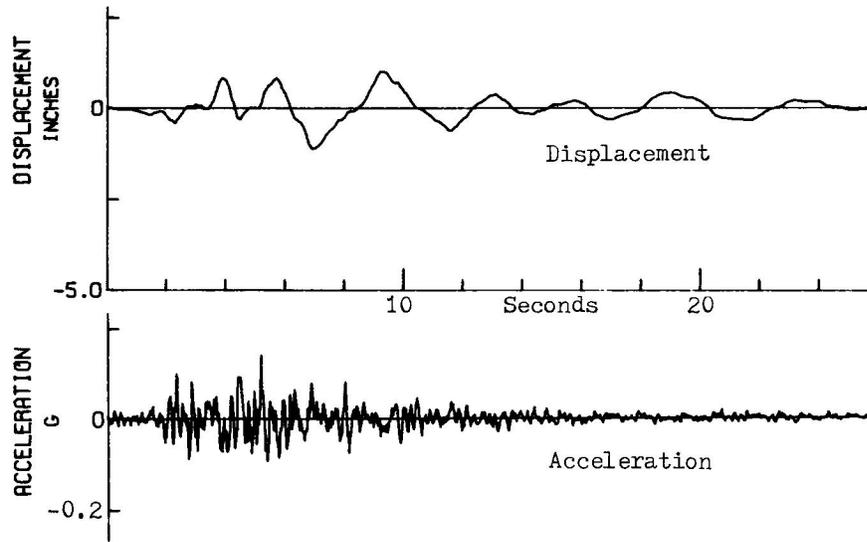
Figure 7c. Motion recorded in the basement of the California Institute of Technology Jet Propulsion Laboratory Building during the 9 February 1971 San Fernando earthquake. The building was located approximately 12 miles from the causative fault of this 6.4 magnitude earthquake.
