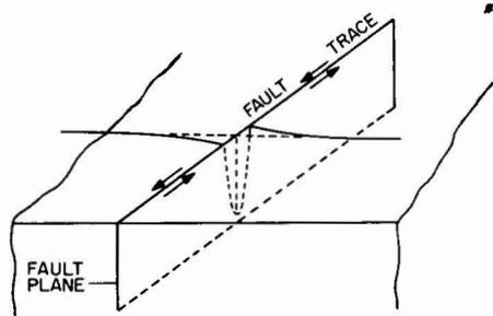
Figure 1c. Strike-slip displacement on a vertical fault plane. Example, San Andreas fault in California, San Francisco earthquake of 18 April 1906; 8.2 magnitude.
