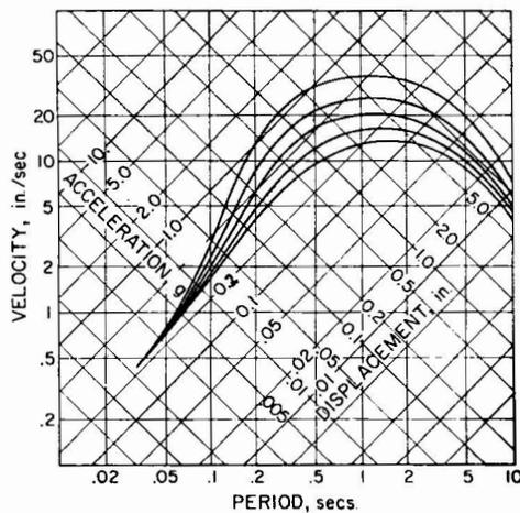
Figure 13. Smooth Design Spectrum from the Response Spectrum of Figure 11. The specification of the design spectrum and the specification of the allowable stresses and strains should be done by the same person who knows what overall strength and what factor of safety the structure should have. (The spectrum curves are for 0, .02, .05, 0.1, 0.2 of critical damping.)
