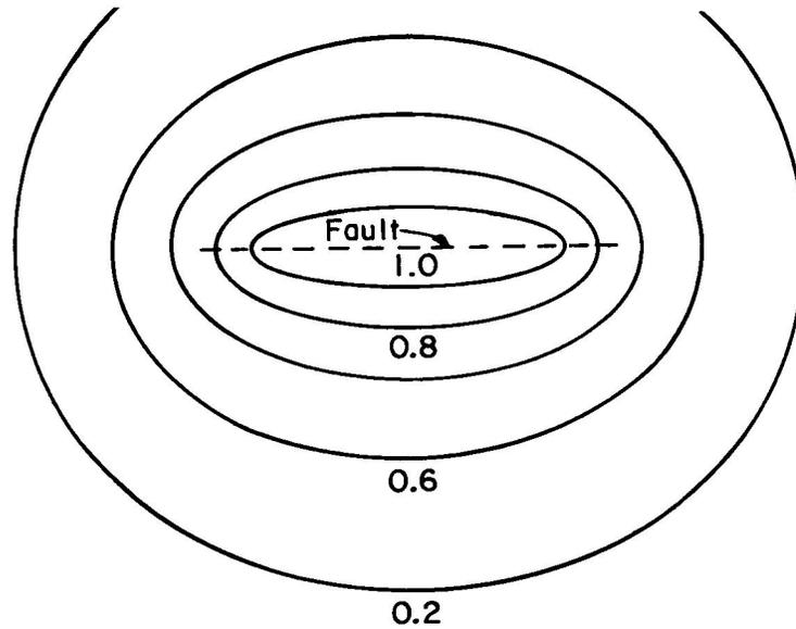
Figure 2. Idealized contour lines of equal intensity of shaking around a causative fault of a magnitude 7.5 earthquake. The contour lines are elongated ovals near the fault but approach circular shapes at large distances. The actual contour lines of an earthquake would be irregular (not smooth) in shape, reflecting nonuniformities in the source mechanism and the geological strata through which the seismic waves travel.
