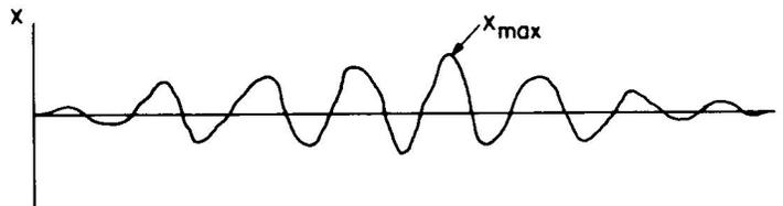
Figure 9. Illustration of the computed displacement of a simple structure of one second period that is subjected to earthquake motion similar to that of the 1972 Managua earthquake.
