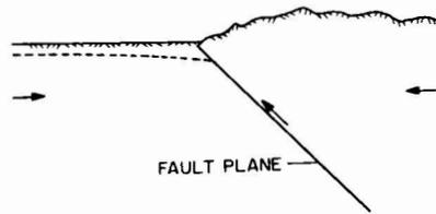
Figure 1a. Thrust faulting under lateral compressive strains. Example, San Fernando, California earthquake of 9 February 1971; 6.4 magnitude.
