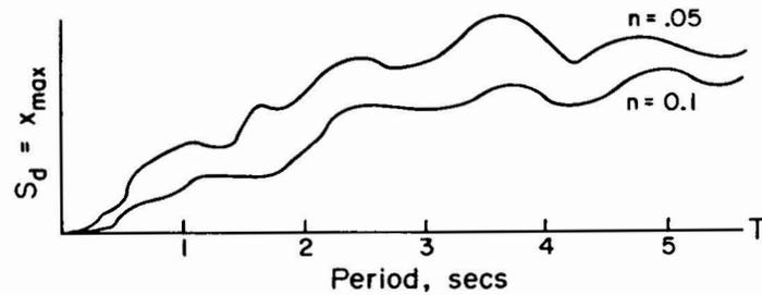
Figure 10. Illustration of Displacement Response Spectrum,  $S_d$ , for two different values of damping,  $n$ . The maximum displacement,  $x_{max}$ , is plotted for a range of periods of vibration.
