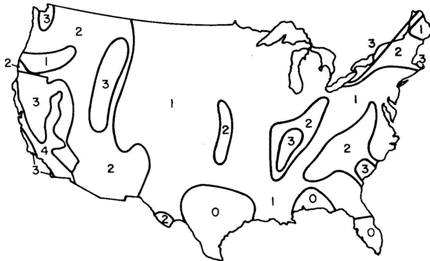
Figure 6. Zoning map that appears in the 1976 Uniform Building Code. The code describes the zones as: Zone 0 - no damage; Zone 1 - minor damage; Zone 2 - moderate damage; Zone 3 - major damage; Zone 4 - indicates Zone 3 regions near major fault systems. The zone numbers determine the seismic forces to be used in design, according to a table provided in the code.
