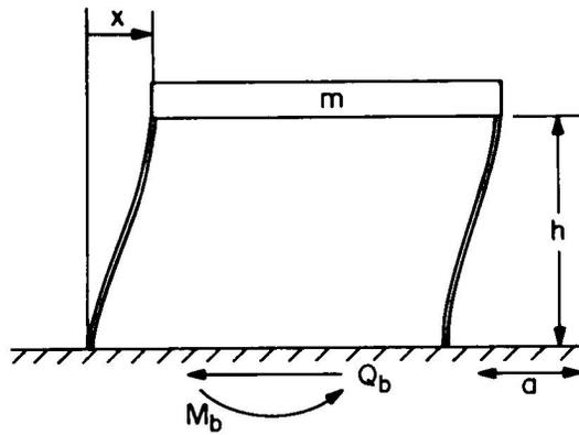
Figure 8. A simple one mass structure having a mass  $m$ , relative displacement  $x$ , story stiffness  $k$ , base shear  $Q_b = kx$ , and base moment  $M_b = h(kx) = hm(\ddot{x} + a)$ . The ground acceleration 'a' causes the structure to vibrate as illustrated in Figure 9.
