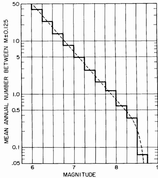
Figure 5. Annual number of earthquakes occurring in the world. The graph gives the expected number having magnitudes between 7.0 and 7.25, and 7.25 and 7.5, etc. The graph is based on the 43 year earthquake record given by Gutenberg and Richter in their book *Seismicity of the Earth*. When plotted on log paper, the data fit closely to a straight line except that beyond  $M = 8.5$  the number of earthquakes falls off, indicating an upper bound.
