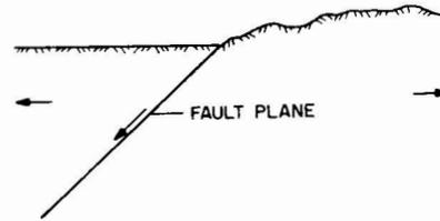
Figure 1b. Normal faulting resulting from lateral extensional strains. Example, Dixie Valley, Nevada earthquake of 16 December 1954; 7.1 magnitude.
